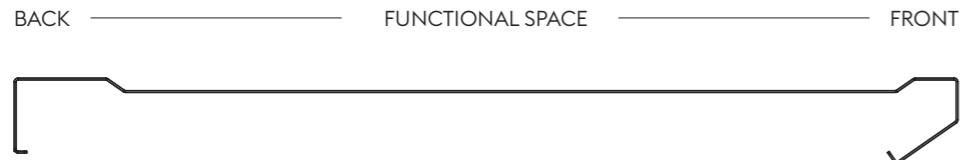
**ENG** Characterised by an unusual and functional profile, the M1 worktop has been designed to simplify the work of every chef and to guarantee the highest level of hygiene. In fact, thanks to the front anti-overflow edge, any liquid or dirt will be contained inside the worktop and will not drip onto the machine and its controls. In addition, a joint gasket has been inserted on the machine sides to retain the same liquids. In this way, an unequalled hygienic barrier is created.
