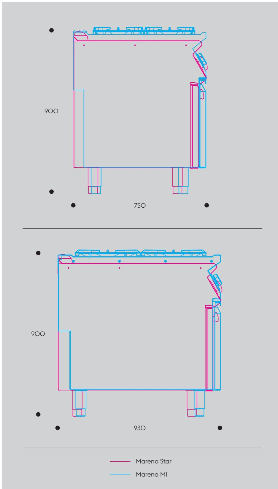
**ENG** Space in the kitchen is important and it is never enough. When designing the M1 range, we chose a solution that would allow you to keep the same footprint, but make the most of the space actually occupied by the machines. So now you can have a wider worktop, brought to a standard height of 900 mm, and more spacious base units, so that you can better organise all the tools you need. Comfort & ergonomics.
